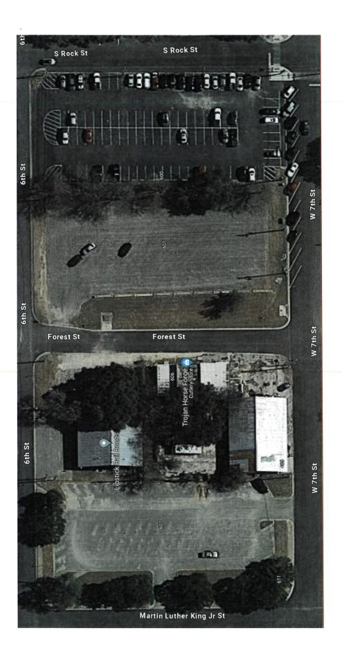
for highways and large paved areas, binder course, 2" thick, and a 6" x 18", includes concrete curb cut for parking lot (601) along with curb stops Scope of work for the Parking lots by the Lip stick Bail Bonds. Parking lot 601 and 600 will get a complete overlay with Plant-mix asphalt paving, and Painted pavement markings, thermoplastic, white or yellow, arrows. Parking lot 607 will have one small repair on the South side of the parking lot.
