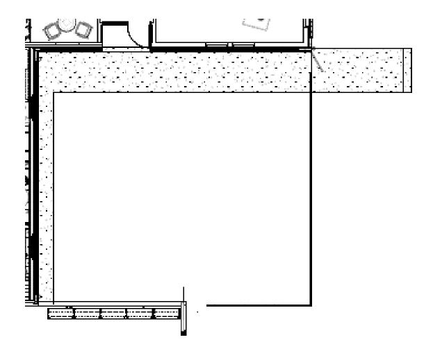
The outdoor area is an 875-square-foot area surrounded by a concrete pathway and a 6-foot wooden fence. The conceptual design is to add a poured-in-place rubberized surface to prevent injuries and a low playground structure for children to engage in play while receiving services related to the disclosures of physical and sexual abuse.
