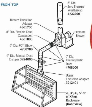
Contact Labconco for ducting options for XPert Enclosures connected to Remote Blower 7068200, 7068300, 7068400 or 7068500. See inside back cover for Typical Exhaust System for 8' XPert Enclosures.
