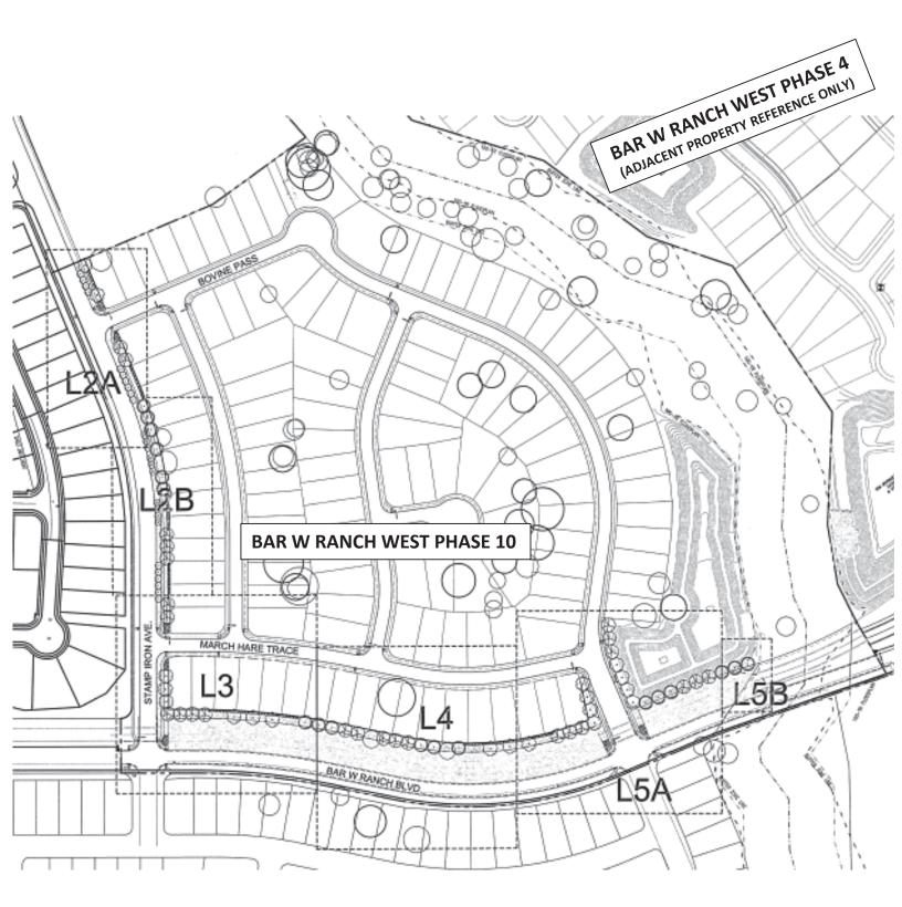
1) No installation of irrigation, plantings, silt fence, etc. shall be permitted within the base overbuild or three feet behind the back of curb.
