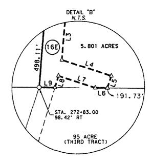
1) All bearings recited herein are based on the Texas State Plane Coordinate System, Central Zone No. 4203, NAD 83. All distances reported hereon are surface values represented in US Survey Feet based on a Grid-to-Surface Combined Adjustment Factor of 1.00014.
